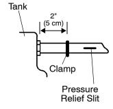
3. Remove the vent line clamp. If the line is bled properly, you should hear a rush of air, indicating that the line is properly primed and ready for operation.
